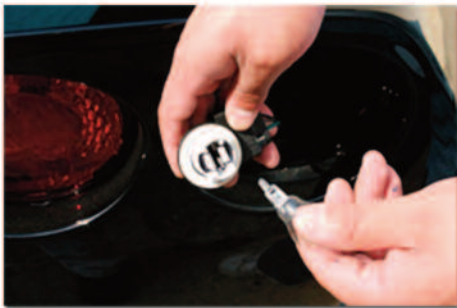
#4- Remove the stock bulb from the socket by pulling it out.
