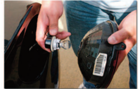
#3- Twist the bulb socket counter clockwise to remove.
