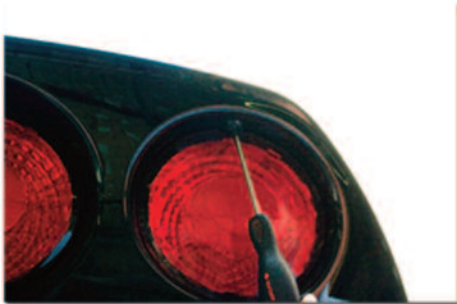
#1- Remove the #15 torx screw at the top of the light.
